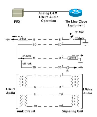
**Note:** For the four—wire audio setup, Pin 6 (Tip) and 3 (Ring) on the router transport the audio path from the PBX to the router. Pin 5 (Tip1) and 4 (Ring1) on the router transport the audio path from the router to the PBX.
