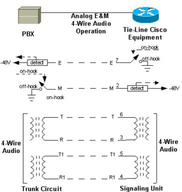
**Note:** For the four—wire audio setup, Pin 6 (Tip) and 3 (Ring) on the router transport the audio path from the PBX to the router. Pin 5 (Tip1) and 4 (Ring1) on the router transport the audio path from the router to the PBX.
