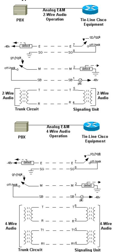
**Note:** For the four—wire audio setup, Pin 6 (Tip) and 3 (Ring) on the router transport the audio path from the PBX to the router. Pin 5 (Tip1) and 4 (Ring1) on the router transport the audio path from the router to the PBX.
