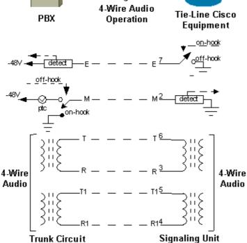
**Note:** For the four—wire audio setup, Pin 6 (Tip) and 3 (Ring) on the router transport the audio path from the PBX to the router. Pin 5 (Tip1) and 4 (Ring 1) on the router transport the audio path from the router to the PBX.
