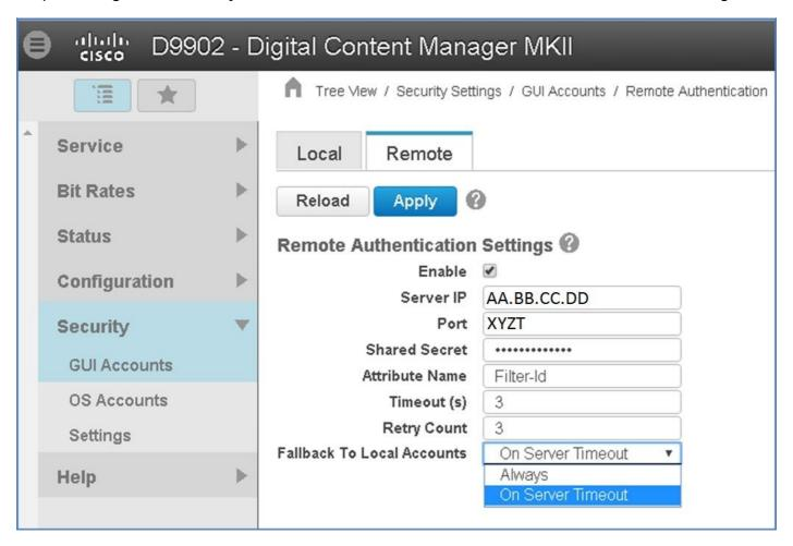
Step 3. Configure the parameters required for RADIUS communication:
