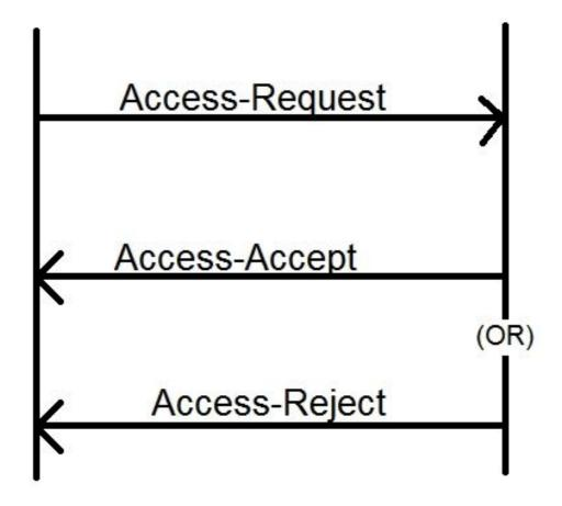
Step 1. User enters the login and password (user account configured on RADIUS server) on the login page on the DCM GUI.
