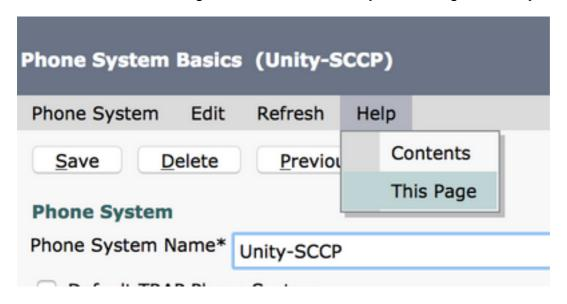
**Step 3.** [Optional] In order to import CUCM users to CUC, configure AXL servers on the Phone System. Navigate to **Edit > Cisco Unified Communications Manager AXL server**.
