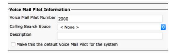
**Step 13.** Configure a Voicemail Profile. The VM Pilot is associated with the VM Profile. Navigate to **Advanced Features > Voicemail > Voicemail Profile** to add a new VM Profile. The VM Profile is associated with a Line Directory Number (DN) on a user's phone. Users can press the message button on the phone to reach Unity Connection.
