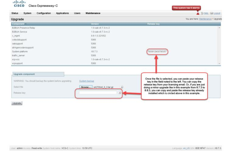
Step 4: Click the **Upgrade** button. Watch the process that follows and do not navigate away from the process, or you have to start over. The image is uploaded, then it is been installed. Click **restart** when prompted.
