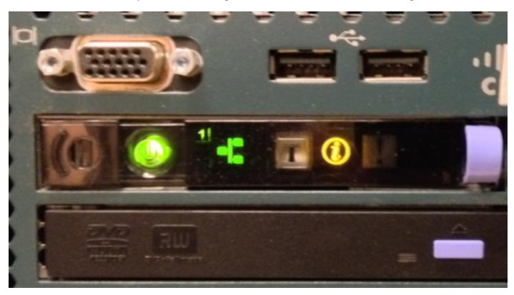
You can see an indicator light turned on when you pull out the panel. In this case, the light is turned on because the system event log is full.
