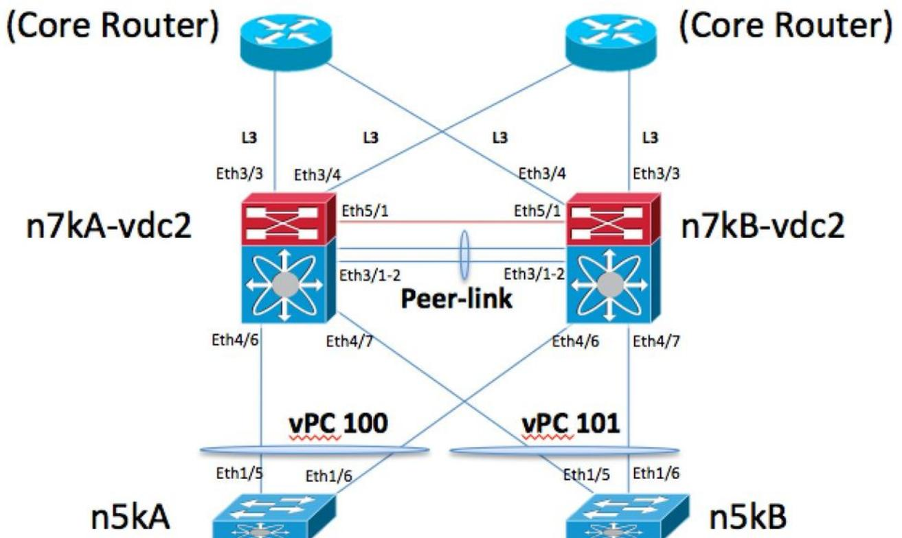
The vPC peer link is Port-channel 1. Ethernet 5/1 is the vPC peer-keepalive link. There are two core routers which are connected via L3 /30 links e3/3 and e3/4 on each N7K box. N5KA and N5KB are simulating L2 switches vPC connected on vPC 100 and vPC 101. N7KA is the vPC primary device.
