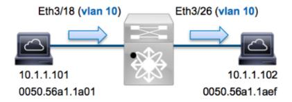
In this example, a host on VLAN 10 (10.1.1.101 with MAC address 0050.56a1.1a01), port Eth3/18 sends an Internet Control Message Protocol (ICMP) request to a host that is also on VLAN 10 (10.1.1.102 with MAC address 0050.56a1.1aef), port Eth3/26. ELAM is used in order to capture this single frame from 10.1.1.101 to 10.1.1.102. It is important to remember that ELAM allows you to capture only a single frame.
