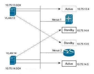
This is an example of HSRP, where there are two routers (Nexus 1 and Nexus 2) and two group users (VLAN 13 and VLAN 14). Through the configuration given below the Nexus 1 is the active router for users in VLAN 13 and standby router for users in VLAN 14; Nexus 2 is active router for users in VLAN 14 and standby router for users in VLAN 13. So the traffic will be shared by these two nexus routers, and also provide first–hop routing redundancy.
