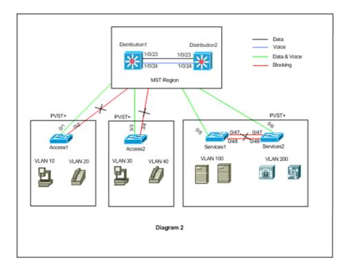
Distribution1 and Distribution2 are in MST region1, and the PVST+ switches see the region1 as a single bridge. The traffic flow after the reconverge is shown in Diagram 2. You can still tune the PVST+ (spanning–tree VLAN X cost) switches to loadbalance the data and voice traffic as per Diagram 1. After you migrate all the other switches as per steps 2 through 4, you get the final spanning tree topology as per Diagram 1.
