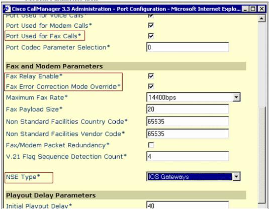
**Note:** This configuration supports voice, Cisco fax relay, and modem pass—through between a VG248, 6608, or 6624 and Cisco IOS gateways (with the exception of the AS5350 and AS5400, which do not support Cisco fax relay).
