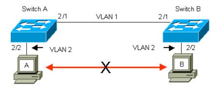
The solution is to enable ISL trunking on the link between switches A and B. Trunking adds a VLAN header to each frame during transmit (multiplex) onto a trunk link. This addition allows the switch at the other end of the link to demultiplex the frames; the switch then forwards the frames to the appropriate VLAN ports.
