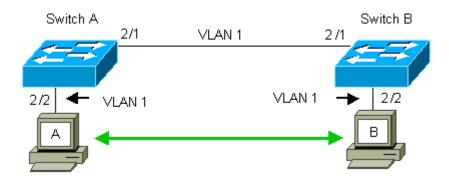
Switches A and B, by default, have the 2/1 ports in VLAN 1. This configuration allows traffic from other ports in VLAN 1 to flow between the switches without the need to configure trunking. References to "the management VLAN" apply to VLAN 1.
