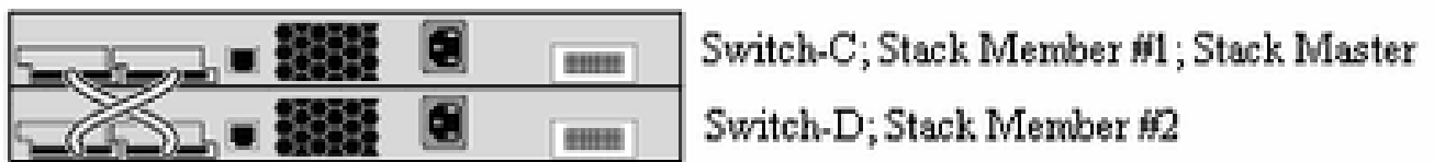
Second Switch Stack Consists of Switch-C and Switch-D
