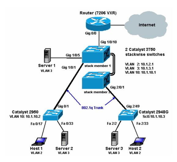
The above diagram shows a small sample network with the stack of Catalyst 3750s providing inter–VLAN routing between the various segments.
