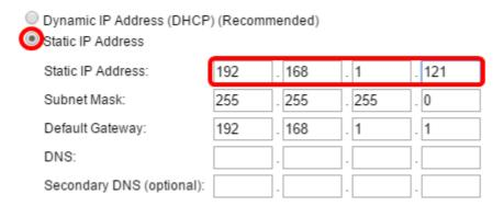
**Note:** In this example, 192.168.1.121 is used as the Static IP Address.
