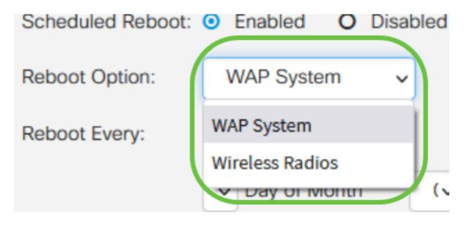
If you notice that the wireless radio is having issues, simply rebooting, and resetting the wireless subsystem during off hours will be faster than a full reboot and might correct any issues you might have.
