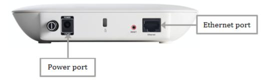
**Note:** Take note of the PoE type that your WAP requires to make sure it is receiving full power supply from your router or switch. Check your devices documentation whether it is capable of 802.3af or the High Power 802.3at PoE standard and verify if your switch or router can provide it to the WAP. To verify PoE power source on your access point, click <a href="here">here</a>.
