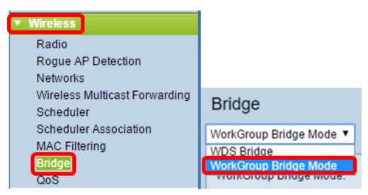
Step 2. Check the **Enable** WorkGroup Bridge Mode check box.
