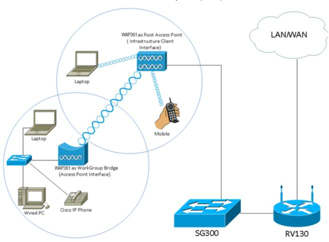
**Note:** The topology above illustrates a sample WorkGroup Bridge model. Wired devices are tethered to a switch, which connects to the LAN interface of the WAP. The WAP acts as an access point interface, connects to the infrastructure interface.
