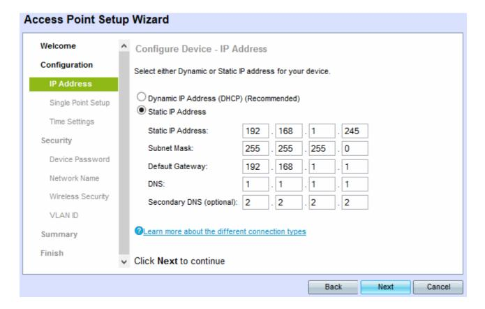
Step 4. Enter the IP address of the WAP in the Static IP Address field. This IP address is created by you and should not be used by another device in the network.
