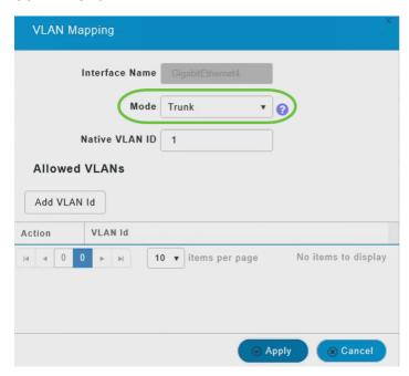
A trunk port can have two or more VLANs configured on the interface; it can carry traffic for several VLANs simultaneously.
