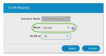
An access port can have only one VLAN configured on the interface; it can carry traffic for only one VLAN.
