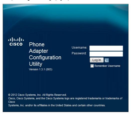
The default IP address of the phone adapter is 192.168.15.1. If no webpage appears try to reset the IP address. In order to reset the IP address, hold the reset button for 30 seconds. This resets the default IP address as well as all other settings to factory defaults. Alternatively, you can manually configure the IP address of the host computer to be on the same subnet as the phone adapter if it is known.
