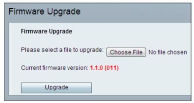
Step 2. Click **Choose File** to choose the firmware version you want to install on the device from where you saved it. Once chosen, the file will appear next to the Choose File button. The Current firmware version field display the current firmware that is installed on the device.
