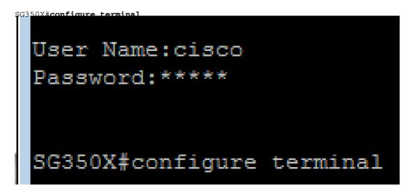
Step 5. By default, SNTP unicast is disabled. Unicast is communication between a single sender and a single receiver. SNTP unicast can be enabled by entering the following command:
