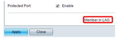
Step 20. Click **Apply**. The port settings are written to the running configuration file. You can then use the Interface field to navigate to a different port to configure its settings, or click **Close** to return to the *Port Settings* page.
