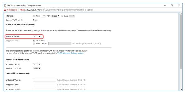
Step 5. Select **User Defined** radio button in the *Tagged VLANs* field. Then enter the VLAN ID's that you want this port to be a member of.
