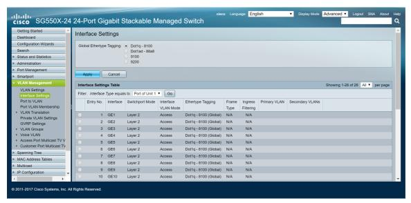
Proceed to configure the same way as: <u>How to Configure Interface Settings on the SG550X-24</u> (<u>active</u>) for both of the non-switches. Configure only the port that is connected to the active switch as trunk port. In this example, GE24 is configured as trunk for both of the switches.
