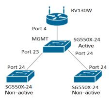
**Note:** The 2 non-active switches are not connected to the active switch until the conclusion.
