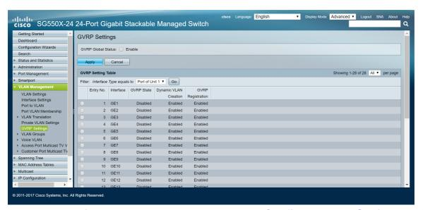
Proceed to configure the same way as the section: <u>Configure GVRP Settings on SG550X-24</u> (<u>active</u>) for both of the non-switches. Configure only the port that is going to be connected to the active SG550X-24 switch. In this example, both of the non-active switch is using port 24 to connect to the active switch.
