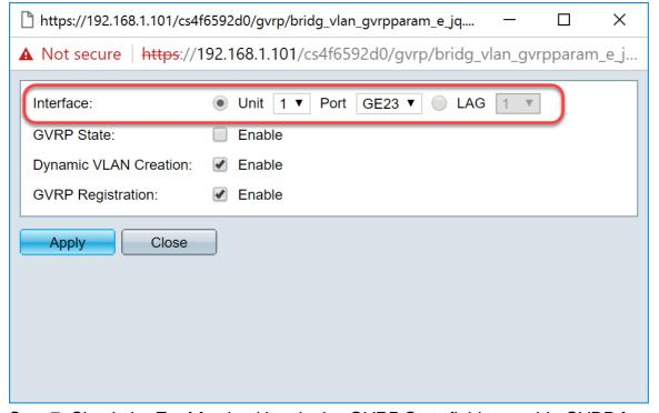
Step 7. Check the **Enable** checkbox in the *GVRP State* field to enable GVRP features on this interface.
