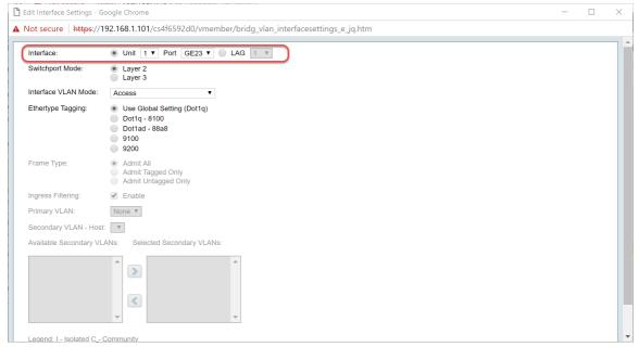
Step 7. Select either Layer 2 or Layer 3 in the Switchport Mode field.
