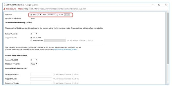
Step 4. When the port is in Trunk mode, it will be a member of this VLAN. Select the **Native VLAN ID** in the *Native VLAN ID* drop-down list.
