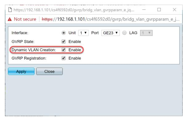
Step 9. (Optional) Check the **Enable** check box in the *GVRP Registration* field to have the selected interface join a VLAN when GVRP information is received for that VLAN on the selected interface. If GVRP registration is disabled, an interface only associates with a VLAN that it is manually configured to be on.
