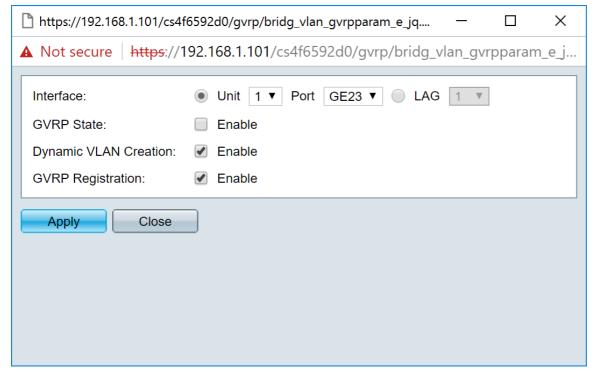
Step 6. (Optional) Click the appropriate radio button and choose a new interface from the Port or Link Aggregation Group (LAG) drop-down list to change the interface whose settings you want to change. LAG bundles individual Ethernet links into a single logical link that can increase the throughput further than a single connection can support.
