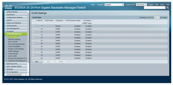
Step 4. Navigate to **Status and Statistics > View Log > RAM Memory** and check to see if GVRP has created VLAN 10-20 for both of the non-active switches.
