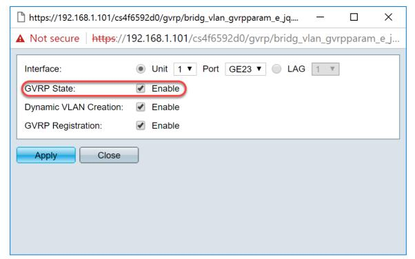
Step 8. Check the **Enable** check box in the *Dynamic VLAN Creation* field to have a VLAN dynamically created if it does not exist when GVRP information is received for that VLAN on the selected interface. If Dynamic VLAN Creation is disabled, the switch only recognizes VLANs that have been manually created.
