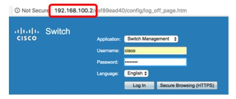
Step 2. Log in to the web-based utility of the switch then choose IP Configuration >IPv4 Management and Interfaces > IPv4 Interface.
