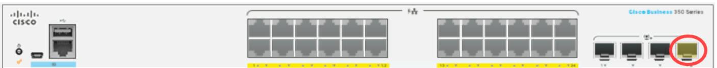
In this example, the cable is connected to XG4 port of the switch.
