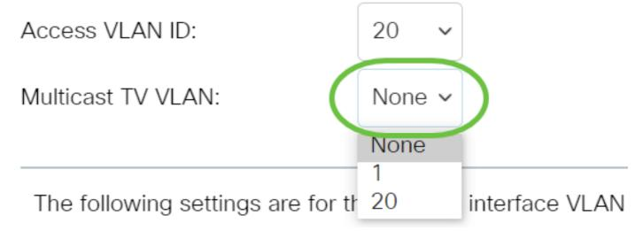
The following settings are for the inactive interface VLAN modes. These effects will be saved, but will not take effect until the interface VLAN mode is changed in the VLAN Interface Settings page. To learn more about how to configure this feature, click <a href="here">here</a> for instructions.
