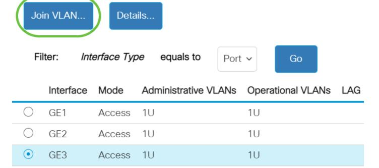
Step 5. Make sure the correct Port or LAG is chosen in the Interface area.
