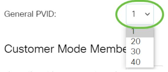
Step 14. (Optional) Choose a VLAN ID from the Customer VLAN ID drop-down list. When the port is in Customer mode, it will be a member of this VLAN.
