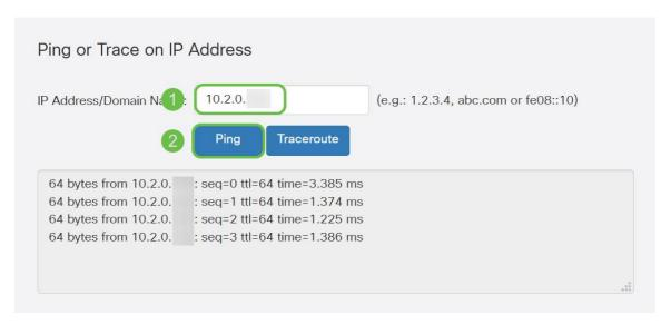
If the ping is successful you will see a message like the above. If the ping fails, it means the DMZ is unable to be reached. Check your DMZ settings to ensure they are configured appropriately.
