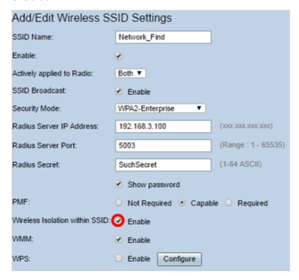
Step 15. Check the **Enable** WMM check box to enable Wi-Fi Multimedia (WMM). This feature allows you to assign different processing priorities to different types of traffic. You can configure Quality of Service (QoS) to provide different priorities and levels of performance to different applications, users, or data flows.
