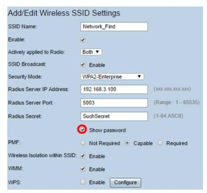
Step 13. Click a radio button in the PMF area to allow Protected Management Frames (PMF) for unicast and multicast frames. The options are:
