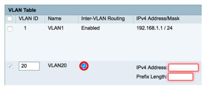
Step 5. In the IPv4 Address field, assign an IPv4 address.
