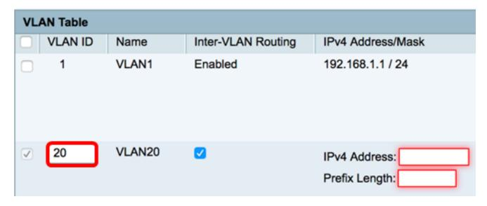
Step 4. (Optional) Check the **Enable Inter-VLAN Routing** check box to allow
