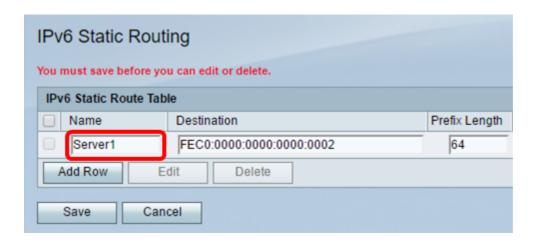
Step 4. Enter the IPv6 address of the destination host or network of the route.
