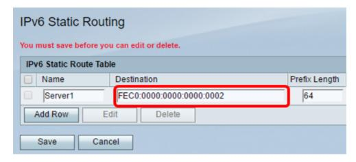
Step 5. Enter the prefix value in bits in the *Prefix Length* field. This is the number of prefix bits in the IPv6 address that define the destination subnet. In this example, 64 is entered.
