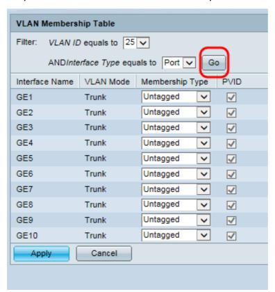
Step 12. For each of the port interfaces of the switch listed in the table, choose the appropriate membership type from the drop-down list. The ports which connect the switch to both the WAP371 (GE1) and the RV130 (GE9) should be Tagged to mark the packets to be identified on the receiving end, while all other unconnected ports for the guest VLAN should be set to Excluded to block guest traffic from entering.
