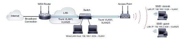
For our scenario, we will have the WAN port of our RV130 plugged in to our broadband Internet connection, and Port 1 on the RV 130 plugged in to port G9 of our SG300. We will also have Port 1 on our SG300 plugged in to the Ethernet port of our WAP371. We will be using the 5GHz band on the WAP371 in order to take advantage of the higher bandwidth.
