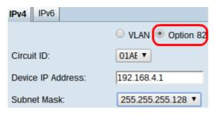
Step 1. Click the **Option 82** radio button to configure DHCP with circuit IDs. Circuit IDs are user specified interface names at which the DHCP client is connected.
