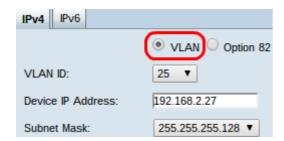
Step 1. Click the **VLAN** radio button to configure DHCP settings for a specific VLAN. Virtual Local Area Networks (VLANs) are networks that are logically divided into different broadcast domains.
