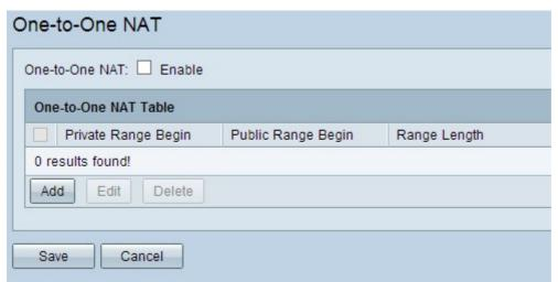
Step 2. Check the **Enable** check box in the *One-to-One NAT* field to enable One-to-One NAT.
