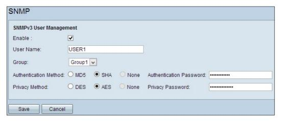
Step 2. Check **Enable** to enable user management for SNMP.
