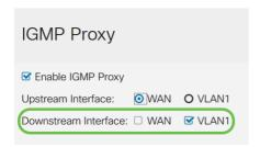
Note: The upstream interface sends out IGMP membership requests on behalf of all the devices on the downstream side of the IGMP Proxy.
