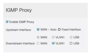
Step 5. Select the *Downstream Interface* from the list to enable the IGMP proxy to receive IGMP membership requests.
