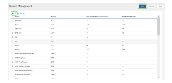
To add a service, click on the *plus icon* and configure *Name, Protocol, Port Start/ICMP Type/IP Protocol and Port End/ICMP Code.*
