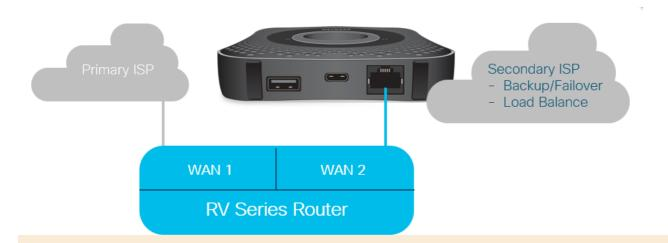
Before connecting the LTE router into the RV340 router, follow the instructions below to set up the LTE router as a backup Internet.
