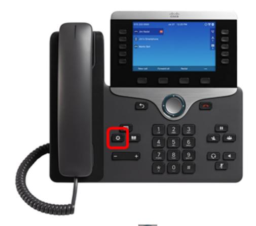
Step 2. Using the Navigation cluster button, navigate to **User preferences** then press the **Select** softkey.
