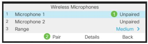
Step 6. Press and hold **Mute** on the wireless microphone until the microphone LED blinks white. If the pairing succeeds, the phone screen displays a success message.
