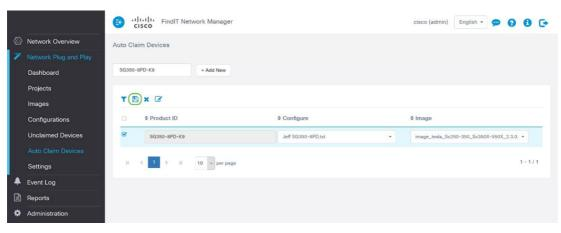
**Note:** Once this action is complete, moving forward, the Network PnP server will use the Image and Configuration to provision any device connecting to the network and matching that PID.
