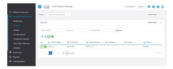
Step 6. Select the **Image** and/or the **Configuration File** you would like automatically applied to this device, complete the provisioning by clicking the **Save Icon**.
