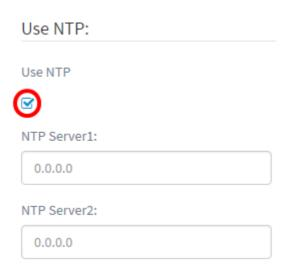
Step 18. In the *NTP Server1* field, enter an NTP server address. A host name can consist of one or more labels, which are sets of up to 63 alphanumeric characters. If a host name includes multiple labels, each is separated by a period. A green checkmark appears in the field if the entered NTP server address is valid.
