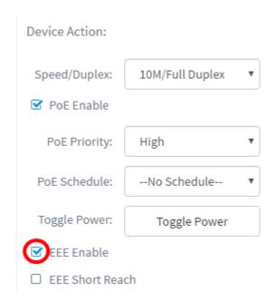
Step 9. Check the **EEE Short Reach** check box to enable EEE Short Reach. This mechanism allows you to run the links with less power than the link can normally handle. It was mainly used in Gigabit Ethernet links due to the limitations of some pluggable modules which had a limit of power it could carry which was less than the normal power, therefore, it became necessary to reduce the power in the gigabit link. This mode is only possible if there are Gigabit Ethernet ports in the switch.
