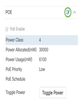
Step 6. Check the **PoE Enable** check box to enable PoE and set the PoE settings below:
