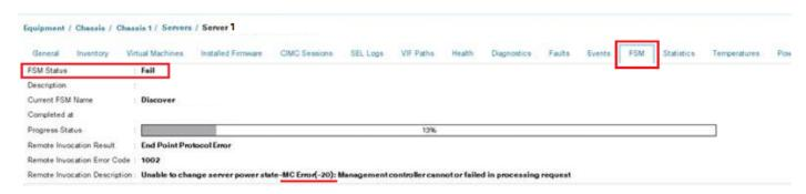
Step 2: Note down impacted blade Serial number and Decommission the Blade.
