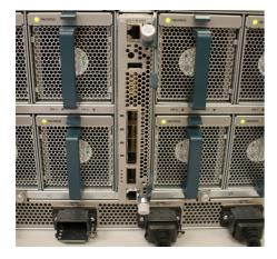
The 40Gbit interface (Scalability Port) can be used with a breakout cable that transforms to 4 x 10Gbit cables.
