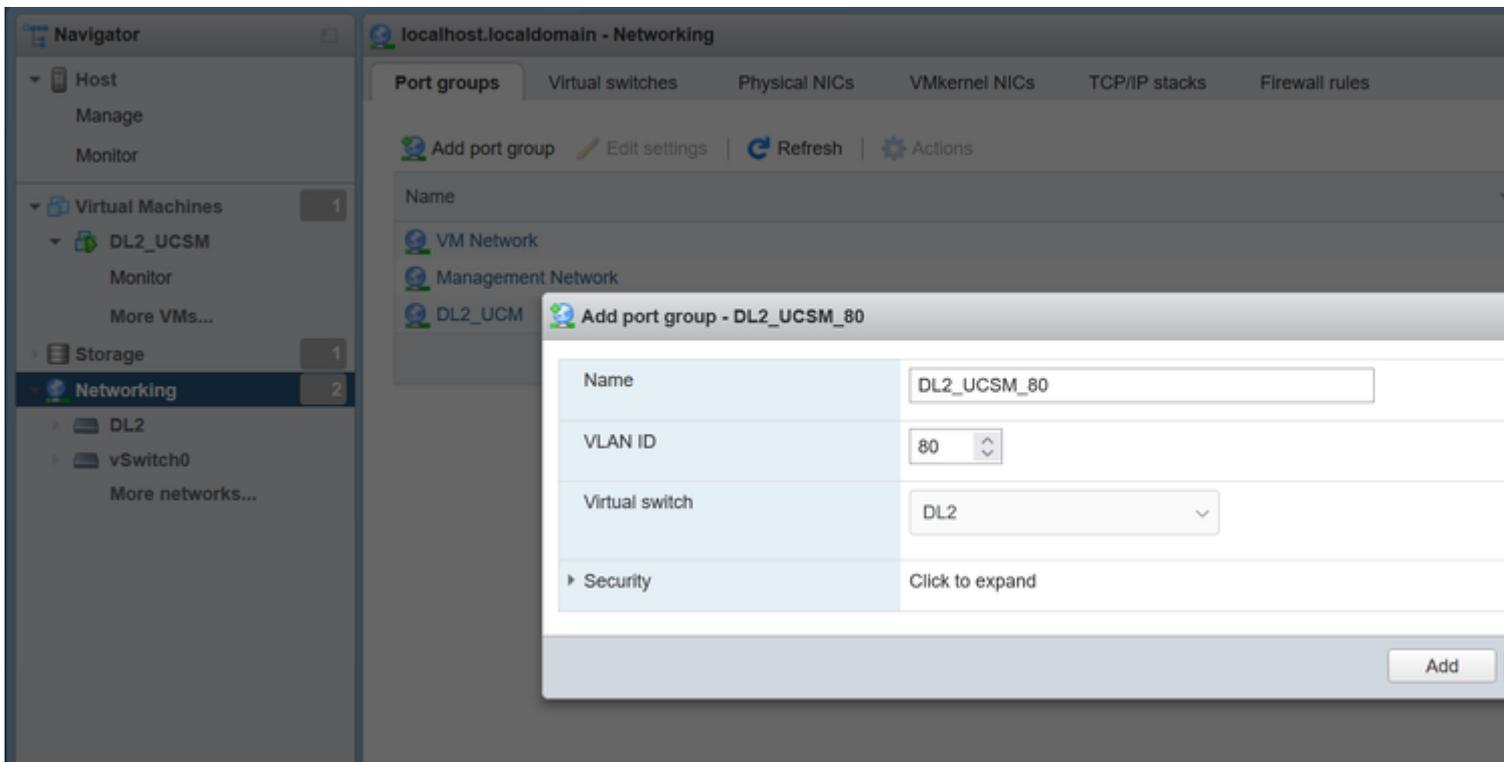
**Step 3.** Navigate to Networking, select the vSwitch previously configured, and click on add uplink. In order to have redundancy add a new uplink that includes the VLAN used for the Disjoint Layer 2.
