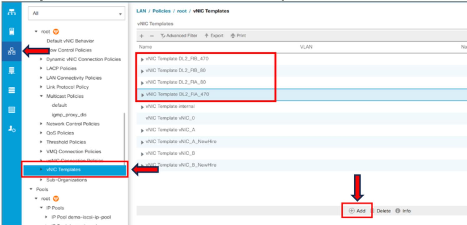
Select the VLANs to be configured accordingly. In this example, the base VLAN is **VLAN 470**, and the disjoint VLAN is **VLAN 80**.
