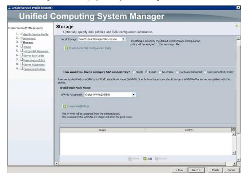
When the Storage section is displayed, complete the configuration as shown here.
