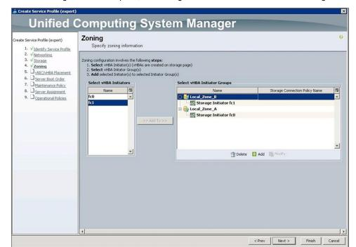
After the configuration is complete, the Zoning window will resemble the screen image shown here.
