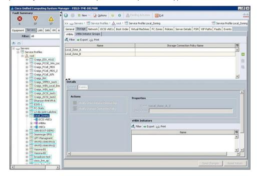
You can view and modify the vHBA Initiator Groups from within this window. To view an existing vHBA Initiator Group, click the name of the group. The details of the vHBA Initiator Group will be displayed in the Details section in the lower part of the screen (use the scroll bar on the right in the Details screen to view the specific Storage Connection Policy details).
