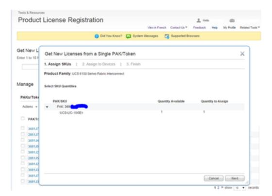
6.The next screen is where the Fabric Interconnect Serial Numbers are inputted, this will transfer that specific license to the Fabric Interconnect Serial Number.
