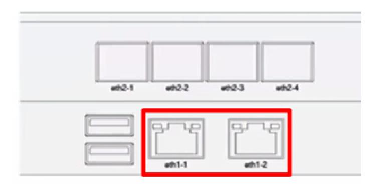
The shared LOM has active/standby mode and active/active mode. It can be changed on CIMC GUI - Admin > Networking > Network (tab) > NIC Properties (section) section. Both active port and the standby port can receive packets, but only the active port can send packets.
